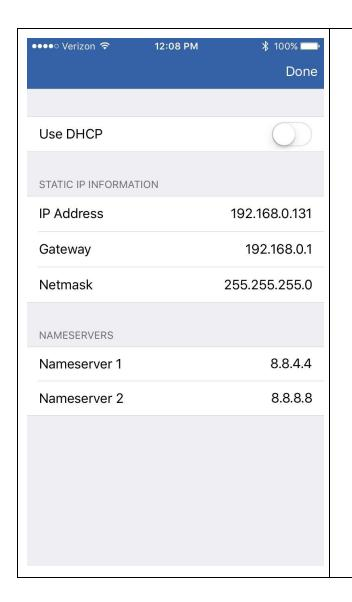
2) To set a static IP address, disable the "Use DHCP" option. Once this option is disabled, you will be able to provide a static IP, netmask and gateway for the router. You can also specify custom name servers at this time. When you are satisfied with your custom network configuration, press the "Done" button.
